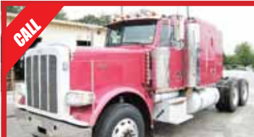
2008 Peterbilt 389 48' Flat Top Sleeper , Cummins 550HP, 18 spd OD, engine brake, air ride, 3.91 ratio, 245" WB, T/A, 12K F/A, 46K R/A, wet line w/P51 pump for walking floor, 528K miles, Stk#751956
