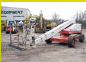
1999 SNORKEL TBA42RDZ: 4,116 HOURS, 42 FT, 4X4, VG RBR, 30" X 60" BASKET, 42 HP DEUTZ DIESEL, ARTICULATING BOOM, ROTATING MAN BASKET, STK#834, $12,500
