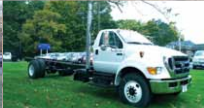
2011 F750 XLT. 6 Spd Automatic, 260" WB, 325HP Cummins, 33,000 GVW
