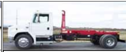
1997 Freightliner FL70 Hooklift, 3126 CAT diesel, automatic, 246,000 miles, new injectors, runs great, 26,000 GVW, new Amprioli A195, 54" Hooklift w/ 18,000LB capacity, $34,500 (file photo), CAREY AUTO, Plympton, MA, 02367, phone 866-637-4076 (rr50eg)
