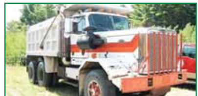
1985 Autocar DK64B, 8 spd, Tandem Axle with a 14 yd body.
