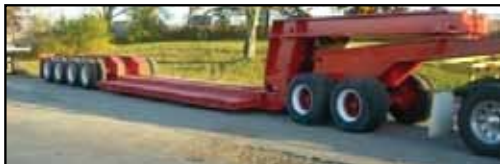
1980 ROGERS 75TON ROGERS LOWBED TRAILER, 24FT DROP SIDE RAIL, 9 WIDE, DETACH FROM BOTH ENDS, 4 axle, T/A Jeep, blasted, prime, & painted.
