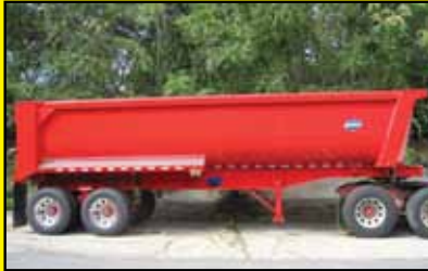
2012 RHODES 30 FT STEEL TRAILER, 70,000# SINGLE POINT SUSP., HIGH LIFT TAIL-GATE, TRI-AXLE PREP. #111135
