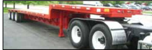
2012 DORSEY 50 TON STEP DECK, 3 AXLE, LIFT IN MIDDLE, HD 8" SIDE RAIL, 6" CROSSMEMBERS, 12" ON CENTER, LED LIGHTS, 255 LO PRO TIRES, CALL FOR MORE INFORMATION.
