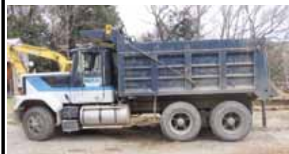
1988 GMC General. CAT 3406B @ 400 H.P., 13 spd., engine brake, 14F+44R on Hendrickson, 11R24.5 steel, 13.6" steel dump. $12,500.
