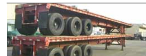
1987 FONTAINE TRI AXLE STRETCH FLATBED TRAILER, EXTENDS FROM 45 X 75. SPRING SUSPENSION, SLIDING AXLES. 2 AVAILABLE TO PICK FROM. CALL FOR MORE INFORMATION.
