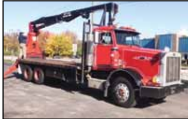
1991 PETERBILT 378 W/PRECAST BOOM AND WIRELESS REMOTE. CUMMINS 370, 9 SPEED, 40,000 LB REARS ON AIR RIDE, 22" STEEL BODY, 102" WIDE, A/C, POWER STEERING, PINTLE HOOK WITH AIR & ELECTRIC. 11 X 22.5 EXCELLENT VIRGIN MATCHED RUBBER, JAKE BRAKE, EXCELLENT SHAPE. OMARK CRANE, MODEL 992158, TYPE PC25 #Z32491. CALL FOR MORE INFORMATION.
