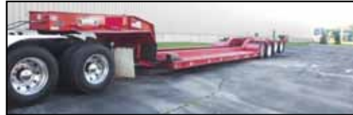
1996 ROGERS 50 TON, 4 AXLE, HEAVY DUTY, CUSTOM DROP SIDE RAIL, 102" WIDE, AIR RIDE, NON GROUND BEARING, LIFT ON 3RD & 4TH PIN ON 4TH 24" DROP SIDE DECK, COMPLETELY RECONDITIONED, SANDBLASTED AND PAINTED, AIR BAGS, BRAKES, SHOCKS, HOSES, EXCELLENT RUBBER 255/70 X 22.5 TUBELESS RADIALS, REGISTERED, WORKING DAILY, HEAVY DUTY SNAP IN OUTRIGGERS.
