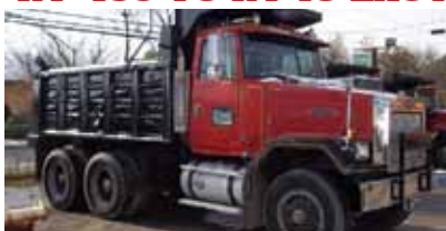
1989 AUTO CAR CUMMINS NTC, 400HP., 301K MILES, 18PSD., 14K FRONT/44 REARS, 4.56 GEARED RATIO, JAKE BRAKE, 24.5 TIRES, 70% TREAD, SINGLE FRAME, HEND. SUSP., AIR BRAKES, A/C, 14FT BEAU ROC STEEL DUMP, AIR GATE, HITCH. $18,000
