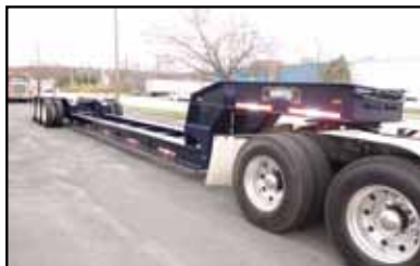
1983 ROGERS 75 TON I-BEAM TRAILER, 3 AXLE, SPRING RIDE, 24" BEAM, HYDRAULIC DETACHABLE, NEW 12 X 24.5 RADIAL TIRES, NEW RIMS, 10" WIDE, DETACHES BOTH ENDS, ONE OWNER, SANDBLASTED, PRIMED & PAINTED, NEW BRAKES, NEW 12 X 24.5 RADIAL TIRES, NEW RIMS, NEW DECALS & DOT TAPE, EXCELLENT SHAPE. CALL FOR MORE INFORMATION.
