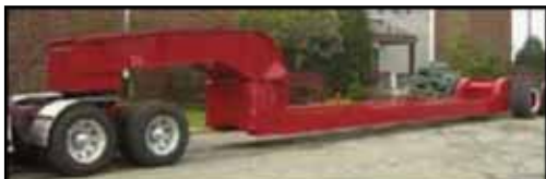
TALBERT 100 TON BEAM TRAILER. 4 Axle, Non Ground Bearing, 29" Deck, Detach both ends, sandblasted, primed and painted, 11 x 24 Rubber, Spring Ride with 4th flip on air. Call for more information.
