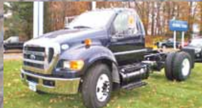
2011 F650 XLT Chassis. 158"WB, Cummins 240HP, Allison 2200 Automatic, 26,000, GVW
