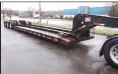
2002 TALBERT 55 TON DROP SIDE RAIL, 26" DECK, 14" LOADED DECK HEIGHT, 102" WIDE, 3 AXLE, AIR RIDE, SET UP FOR 4TH, LIFT ON 3RD, NON GROUND BEARING, 2 PIN POSITION ON GOOSE NECK, VERY LOW MILES, ONE OWNER, EXCELLENT SHAPE. CALL FOR MORE INFORMATION.
