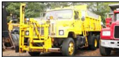
1997 International Tandem axle dump Cummins, automatic, central hydraulics, double wing, former municipal truck, snow ready, $12,500 860-280-4140 (jb50eg)
