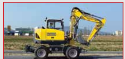
WACKER NEUSON 9503 WHEELED EXCAVATOR, 9.5 Metric Tons, 13' Digging Depth, Rear Blade, 25 MPH, Proportional Control Auxiliary Hydraulics, 100HP Deutz Diesel
