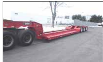
1989 ROGERS HEAVY DUTY 50 TON DROP SIDE TRAILER. HYDRAULIC DETACHABLE, AIR RIDE, LIFT ON 3RD, 102" WIDE, 24" STEEL DECK, LO PRO TUBELESS RUBBER, OUTRIGGERS. SANDBLASTED AND PAINTED, NEW BRAKES, NEW STICKERS, NEW FLAPS. ONE OWNER. CALL FOR MORE INFORMATION.
