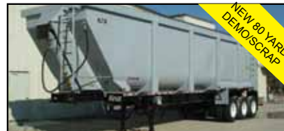
KRUZ 38' X 102" DEMO/SCRAP TRAILER, TRI AXLE, 80 YD, 89" SIDES, 1/4" HARDOX 450, HUB PILOTED WHEELS, TIRE CARRIER, AIR RIDE OR SPRING AVAILABLE. WE TAKE CUSTOM ORDERS ON KRUZ AND TERMINATOR DUMP TRAILERS
