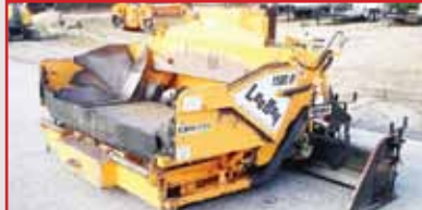
2004 LEEBOY 1000D, 36HP, Legend Screed 8-13' propane, 6-Ton hopper, steel tracks, Hatz 2L41C engine, $26,000
