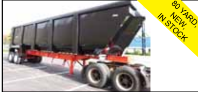
2013 KRUZ 38' STEEL DEMO TRAILER. 2 AXLE, 70,000 LB SINGLE PT SUSP, 11 X 24.5 TIRES, HOLLAND MARK V LANDING GEAR, HARDOX 450 STEEL, 9 PANEL GATE. CALL FOR MORE INFORMATION.
