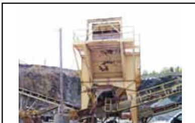
ALLIS 8 X 20 TRIPLE DECK INCLINED SCREENING PLANT WITH THREE DECKS OF FLEX MAT SCREEN MEDIA INSTALLED SUPER STRUCTURE, CHUTES, ACCESS LADDERS, CAT WALKS.
