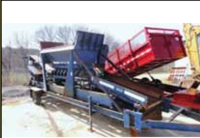
RAWSON SCREENING PLANT, MODEL 3618, 3 YD. CAPACITY, REMOTE DUMPING GRIZZLY, EXTRA SCREEN, COMPLETELY REFURBISHED AT RAWSON FACTORY, WORK READY ! $27,900
