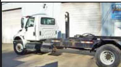
2004 International 4600 Hook-Lift, DT466, auto, 26,000 LB GVW, air brakes, air ride, 54" Hook, 20,000 LB K-Pac Hoist, loaded.
