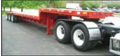
2013 DORSEY 50 TON STEP DECK, 3 AXLE, LIFT IN MIDDLE, HD 8" SIDE RAIL, 6" CROSSMEMBERS, 12" ON CENTER, LED LIGHTS, 255 LO PRO TIRES, CALL FOR MORE INFORMATION.
