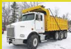
1997 KENWORTH T800: TRIAXLE, 17 FT STEEL A/C, HITCH, NO AIR, CUMMINS L10, 300 HP, 8LL, HEND. SPRING SUSP., 46K R, 20K F, 15K TAG, STK#715, $29,500
