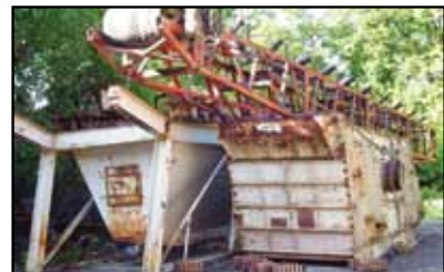
DIESTER 6 X 16 TRIPLE DECK INCLINED SCREENING PLANT WITH SUPER STRUCTURE, CHUTES, ACCESS LADDERS, CATWALKS AND STANTION.
