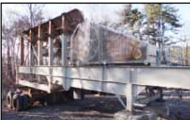
CEDAR RAPIDS, 30 X 54 PORTABLE JAW PLANT WITH ROCK CRUSHING NIP ANGLE INCLUDES ROCK HOPPER WITH SUPER STRUCTURE, CHUTES, GUARDING, CATWALKS, ACCESS LADDERS AND CONTROL HOUSE.
