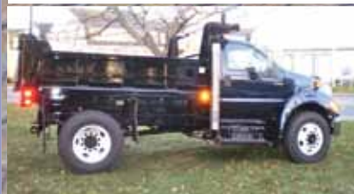
2011 F650 XLT DUMP BODY. Cummins 240 HP, Allison 2200 Automatic, 26,000 GVW
