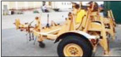
USED 1993 BUTLER REEL/SPOOL TRAILER , SURGE BRAKES, HAND OPERATED HYDRAULICS TO LIFT REEL FROM GROUND, A DISC BRAKE TO STOP FROM UNWINDING. AS IS $3,900. WRIGHT TRAILERS, INC. 508-336-8530
