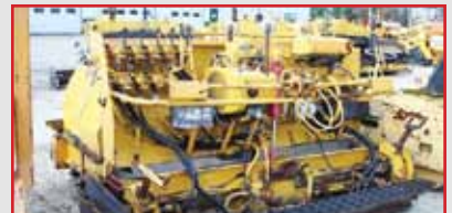
1989 MAULDIN 550, Kohler gas, 23 hp, Screed 8-12ft propane, Rubber tire, Dump hopper, $3,500
