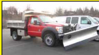
2012 Ford F550 XL 9' Aluminum dump body, 9' Fisher stainless steel plow, diesel, 4x4, power group, #125109
