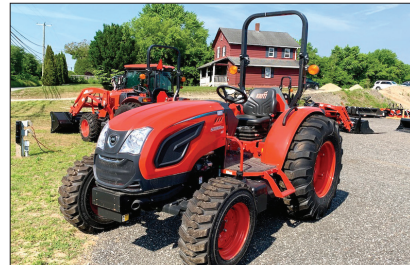
KIOTI DK5310HSE Tractor w KL5521 Loader, 66" Bucket, 50.3HP, 3 Range HST Trans., 2,716Lb. Lift Capacity, $33,988
